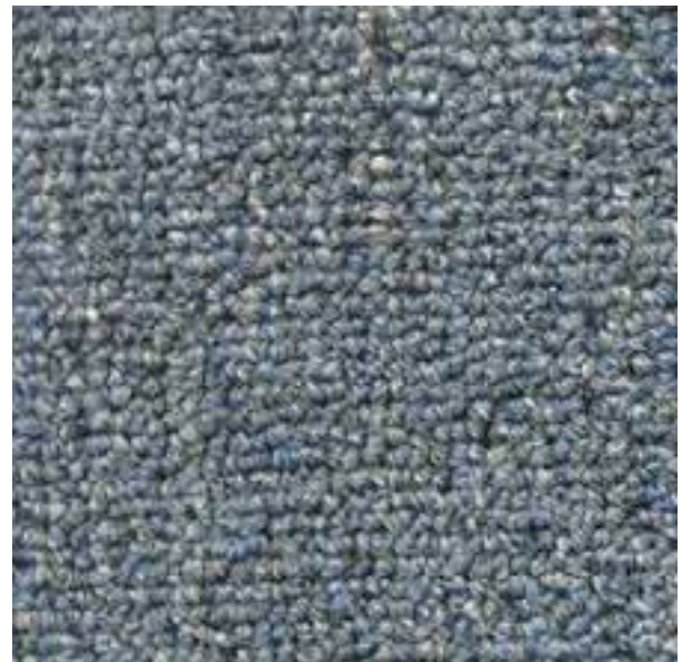
Olefin level loop commercial carpet most often installed by direct glue down method
