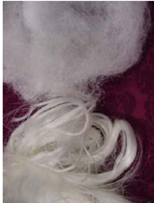
-Crimped and uncrimped fibers compared
